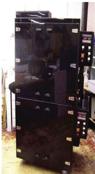
FIGURE 1 | The completed light:dark chamber, which consists of two separate units.
